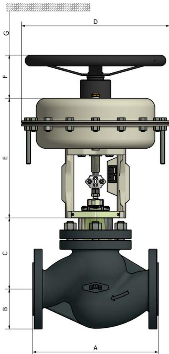
(\*) According to standard EN1092-1 DN65 valves in carbon steel and stainless steel flanged PN16 must be provided with 8 holes. They can be supplied with 4 holes only at the specific request of the customer.
