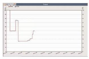
A deviation time out alarm occurs when the difference between the target position and the actual position exceeds the preset deviation alarm point (for more than the preset deviation time).
